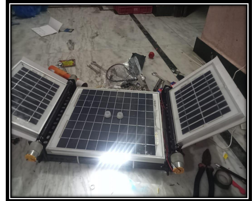
Design and Fabrication of two fold Adjustable Solar panel External attachment on the top of E-Vehicle for charging Battery
